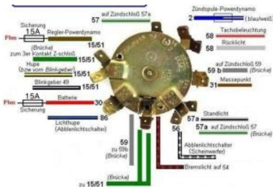
Wiring of the ignition lock for the new system.
